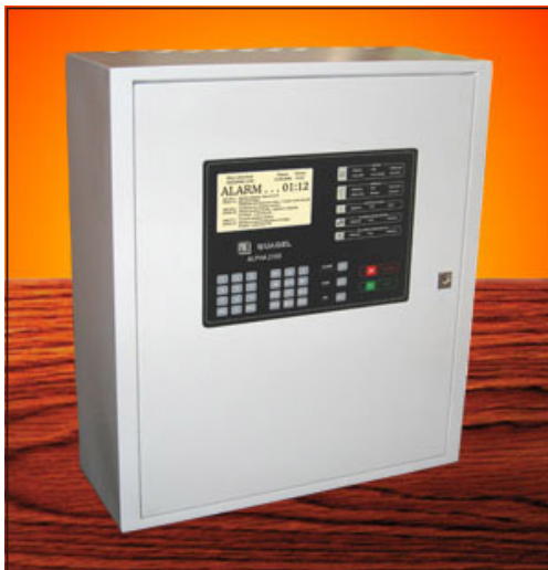
Figure 6. Alarm central station [3]
